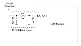
Figure 16: Reference Design for Active Antenna
