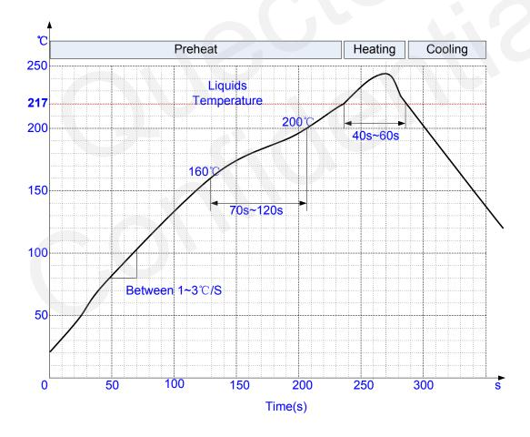
Figure 23: Ramp-soak-spike-reflow of Furnace Temperature
