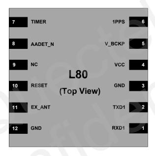
Figure 2: Pin Assignment
