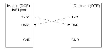
Figure 12: Connection of Serial Interfaces
