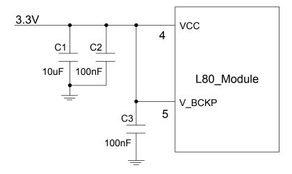
Figure 4: Reference Circuit for Power Supply
