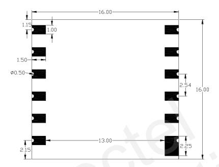
Figure 19: Bottom Dimension (Unit: mm)
