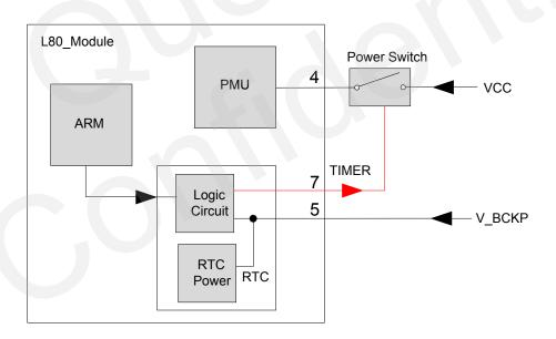
**Figure 3: Internal Power Construction**
