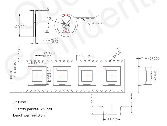
Figure 24: Tape and Reel Specification
