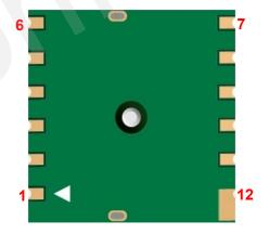
Figure 22: Bottom View of the Module
