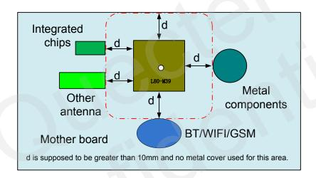
Figure 15: L80 Module Placement Guide
