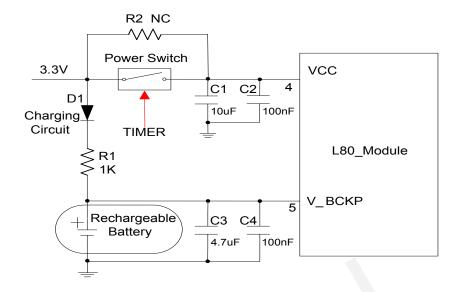
Figure 5: Reference Charging Circuit for Chargeable Battery
